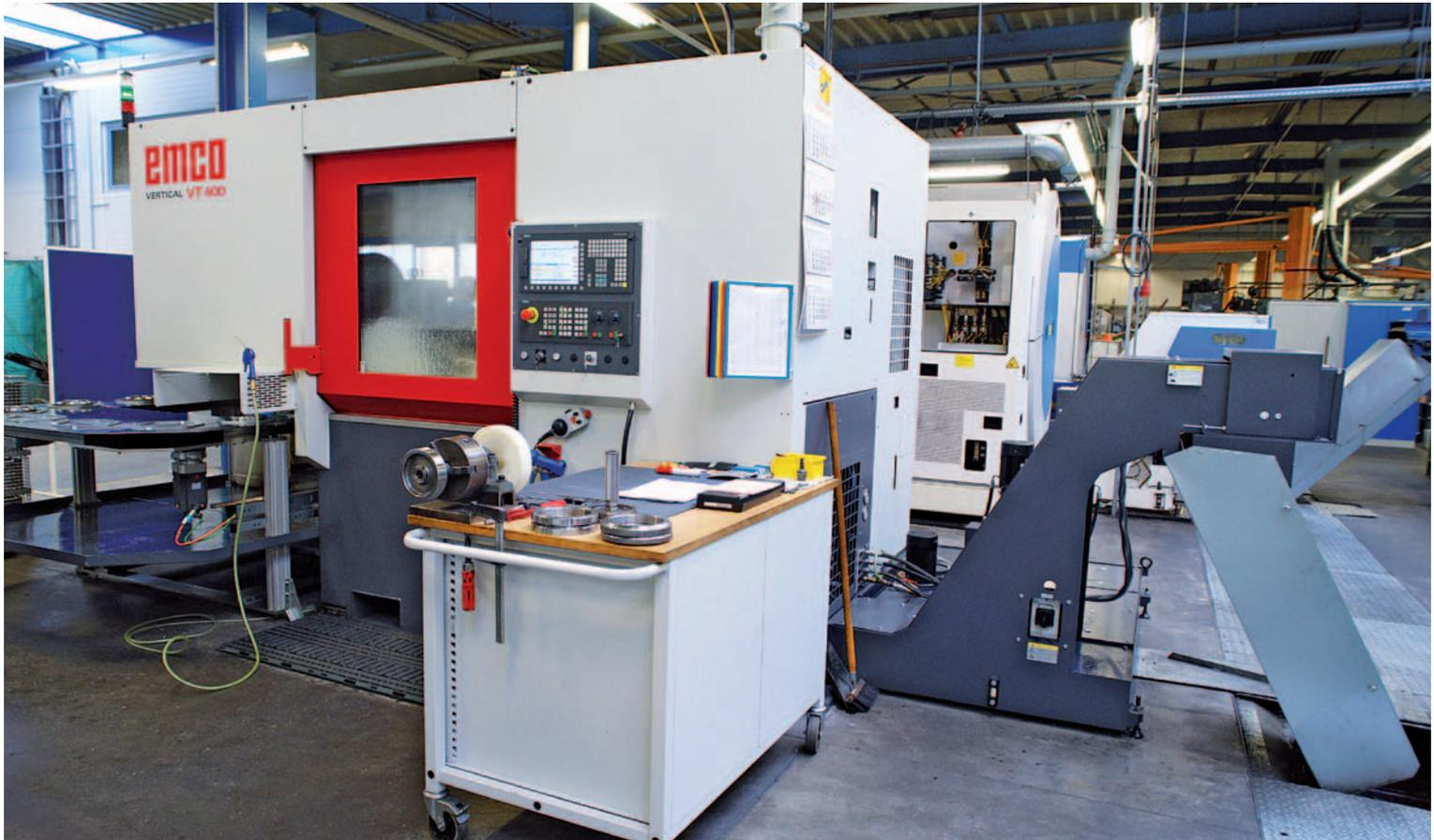
On the left of the VERTICAL VT 400, the drag frame belt conveys the parts that are to be processed, as well as those which have been completed; on the right is the central chip disposal.
